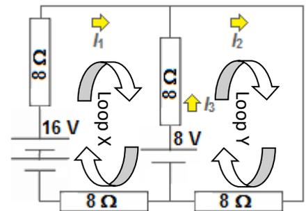
29. Find the values of the three currents and the four resistor voltages. Write them in the diagram.
