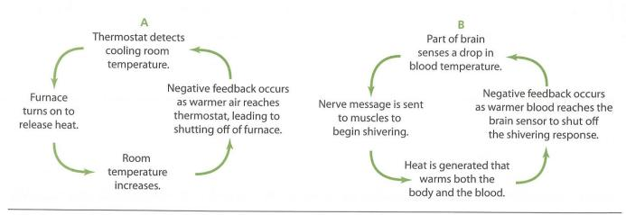
Figure 2-10. Negative feedback systems: (A) The furnace and thermostat in most houses are part of a negative feedback system.
