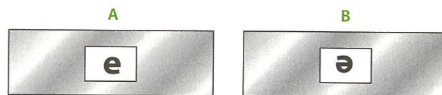
Figure 9-10. Microscope view: The letter “e” as seen on a slide (A) and as seen through the microscope (B). (Only the change in position of the letter is shown, not magnification.)
