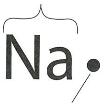
Figure 6-2. The Lewis dot diagram of a sodium atom: The kernel, represented by the symbol Na, contains 11 protons and 10 electrons; the kernel has a 1+ overall charge. The 1+ charge of the kernel is balanced by the 1- charge of the single valence electron. Overall, the sodium atom is neutral.
